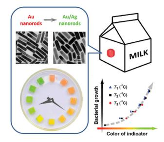
Fig. 9 A kinetically programmable time-temperature indicator. (Left) Chronochromism during the overgrowth of the silver shell layer on gold nanorods. (Bottom right) A temperature-independent correlation between the indicator color and the magnitude of microbial growth in perishable.
