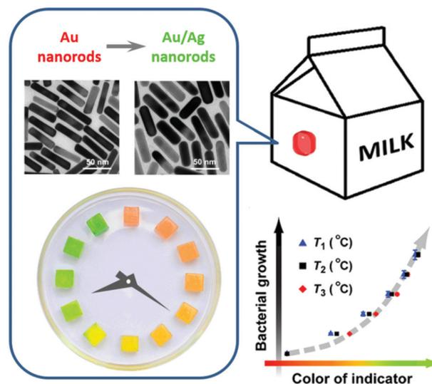
**Fig. 9** A kinetically programmable time-temperature indicator. (Left) Chronochromism during the overgrowth of the silver shell layer on gold nanorods. (Bottom right) A temperature-independent correlation between the indicator color and the magnitude of microbial growth in perishable.
