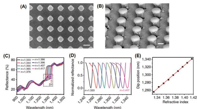
**Fig. 2** Sensing platform comprising gold mushroom arrays. (A, B) Scanning electron microscopy images of gold mushroom arrays. (C) Reflectance spectra of gold mushroom arrays immersed in solutions with varying refractive indexes ( $n$ ). (D) Spectral profiles for D1 after normalization. (E) The linear correlation between the dip wavelength and the refractive index (reprinted with permission from ref. 67).
