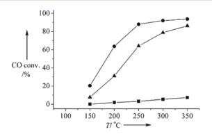
Fig. 9 WGS reaction "light-off" profiles for 1% Au on CeO2 nanorods (●), cubes (■), and polyhedra (▲) (modified with permission from ref. 37, copyright 2008 Wiley-VCH).
