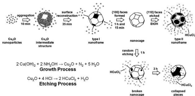
Scheme 4 Schematic illustration of the growth and etching mechanisms in the synthesis of  $\text{Cu}_2\text{O}$  nanoframes and nanocages (modified with the permission from ref. 80, copyright 2008 American Chemical Society).
