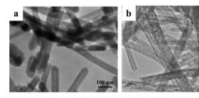
Fig. 2 TEM images of (a)  $Ce(OH)_3$  nanotubes synthesized at 120 °C, (b)  $CeO_2$  nanotubes formed during controlled annealing of the  $Ce(OH)_3$  nanotubes synthesized at 120 °C (modified with permission from ref. 60, copyright 2005 Wiley-VCH).
