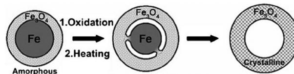
**Scheme 6** Synthesis of core-shell-void  $\text{Fe}-\text{Fe}_3\text{O}_4$  and hollow  $\text{Fe}_3\text{O}_4$  nanoparticles from  $\text{Fe}-\text{Fe}_3\text{O}_4$  nanoparticle seeds (modified with permission from ref. 84, copyright 2007 Wiley-VCH).
