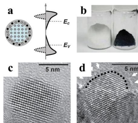
**Fig. 10** (a) Scheme of the structure and band gap of TiO<sub>2</sub> black; (b) photographs of TiO<sub>2</sub> white (left) and TiO<sub>2</sub> black (right) samples; High Resolution Transmission Electron Microscopy (HRTEM) images of (c) anatase NCs and (d) TiO<sub>2</sub> black (modified with permission from ref. 104, copyright 2011 American Association for the Advancement of Science).
