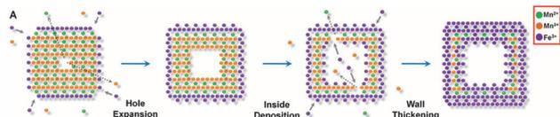
**Scheme 5** Schematic illustration of the transformation of  $\text{Mn}_3\text{O}_4$  NCs, showing the evolution of their morphology via the localized dissolution of  $\text{Mn}_3\text{O}_4$  and the surface precipitation of  $\gamma\text{-Fe}_2\text{O}_3$  (modified with permission from ref. 82, copyright 2013 by the American Association for the Advancement of Science).
