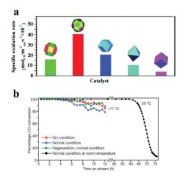
Fig. 8 (a) Specific oxidation rates of the CO oxidation reaction on various shaped Cu<sub>2</sub>O microcrystals (modified with permission from ref. 38, copyright 2010 American Chemical Society); (b) CO oxidation stability test of Co<sub>3</sub>O<sub>4</sub> nanorods under stream under different conditions (modified with permission from ref. 22, copyright 2009 Nature Publishing Group).
