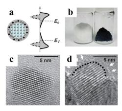
Fig. 10 (a) Scheme of the structure and band gap of TiO<sub>2</sub> black; (b) photographs of TiO2 white (left) and TiO2 black (right) samples; High Resolution Transmission Electron Microscopy (HRTEM) images of (c) anatase NCs and (d) TiO<sub>2</sub> black (modified with permission from ref. 104, copyright 2011 American Association for the Advancement of Science).
