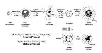
Scheme 4 Schematic illustration of the growth and etching mechanisms in the synthesis of Cu<sub>2</sub>O nanoframes and nanocages (modified with the permission from ref. 80, copyright 2008 American Chemical Society).
