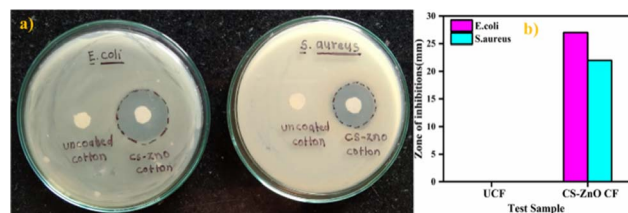
Fig. 7 (a) and (b) Antibacterial activity of UCF and CS-ZnO CF against E. coli and S. aureus .
