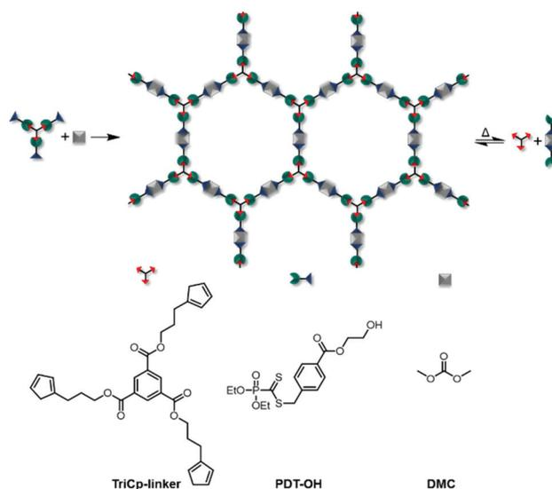
**Scheme 1** General concept of the bonding/debonding on demand polycarbonate. The network is formed *via* the reaction of a triol species (**HDA-triol**) – which is formed *via* an HDA reaction of the **TriCp-linker** and **PDT-OH** – with dimethylcarbonate using TBD as catalyst. The network is then able to bond and debond on demand due to the HDA units within minutes as a function of the applied temperature.
