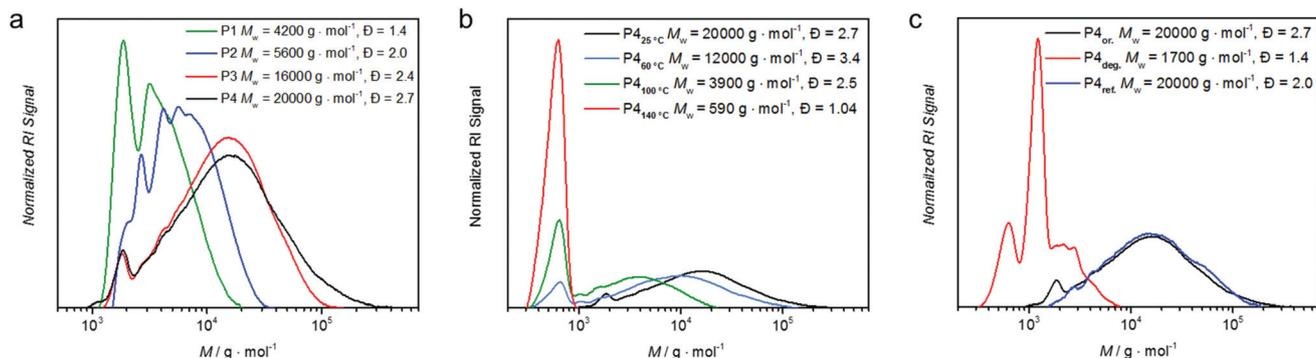
**Fig. 1** Analysis of the bonding/debonding behavior of the HDA-containing linear polycarbonates. (a) SEC analysis of polycarbonates P1–P4 with different degrees of polymerization. (b) SEC analysis of P4 at 25, 60, 100 and 140 °C. (c) SEC analysis of the bonding/debonding behavior of P4 upon heating and cooling. P4<sub>or</sub> is the original P4 polymer, P4<sub>deg</sub> the degraded polymer at 120 °C and P4<sub>ref</sub> the reformed polymer upon cooling. Solvent: THF.
