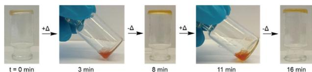
**Fig. 3** Bonding/debonding behavior of the prepared HDA-containing polycarbonate network (+ $\Delta$ : heating to 120 °C,  $-\Delta$ : cooling to 25 °C). Heating was conducted with a preheated oil bath and a water bath was used for cooling. The time indicates the minute, at which the picture was taken. The red color upon heating is due to the formation of a dithioester species (rHDA1).
