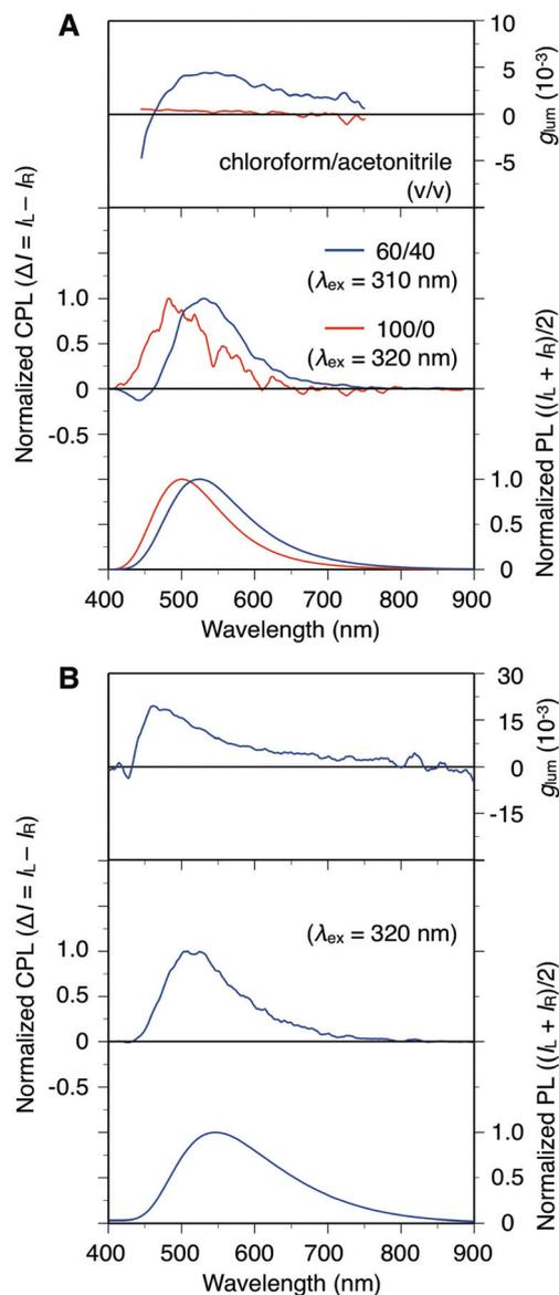
Fig. 5 PL (bottom), CPL (middle) and  $g_{lum}$  (top) spectra of poly-9 ( $1.0 \times 10^{-4}$  M) in chloroform/acetonitrile (100/0 or 60/40, v/v) (A) and of a chloroform-cast film of poly-9 after exposure to acetonitrile vapor for 96 h (B) at room temperature. The corresponding PL (not normalized) and CPL (unprocessed) spectra are shown in Fig. S14.†
