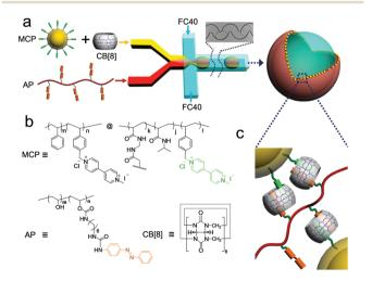
Fig. 2 (a) Schematic of the preparation of supramolecular colloidal microcapsules by a flow-focusing microfluidic device, consisting of a continuous FC-40 oil phase perpendicular to a combination of two aqueous solutions of MCP⊂CB[8] and AP as the dispersed phase. (b) Molecular structure of MCP, AP, and CB[8]. (c) Schematic representation of the proposed microcapsule from CB[8]-mediated supramolecular assembly.
