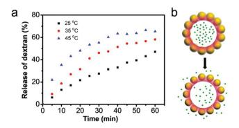
Fig. 7 (a) The release profiles of 150 kDa FD cargo from microcapsules over 1 h, at temperatures: 25, 35 and 45  $^{\circ}$ C. (b) Schematic representation of the contraction of the colloidal particles upon increasing temperature, resulting in release of encapsulated cargo.
