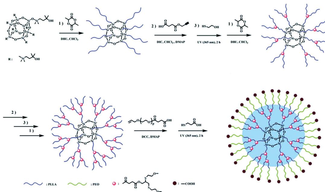
Fig. 6 Schematic illustration of the synthetic route to the core-shell structural amphiphilic copolymer POSS-(G<sub>3</sub>-PLLA-*b*-PEO-COOH)<sub>8</sub> and the unimolecular micelle formation formed from the copolymer. Reproduced with permission from Royal Society of Chemistry.<sup>101</sup>
