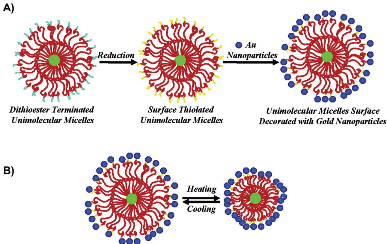
**Fig. 20** (A) Schematic illustration of the two-step preparation of the hybrid unimolecular micelle surface decorated with Au nanoparticles and (B) the thermo-tunable spatial distance between Au nanoparticles attached at the unimolecular micelle surface. Reproduced with permission from American Chemical Society.<sup>203</sup>
