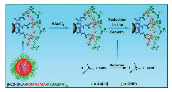
Fig. 19 Schematic representation of using the star-like block copolymer  $\beta$ -CD-(PLA-PDMAEMA-PEtOxMA)<sub>21</sub> as a unimolecular micelle template for the synthesis and stabilization of gold nanoparticles. Reproduced with permission from Wiley.<sup>201</sup>
