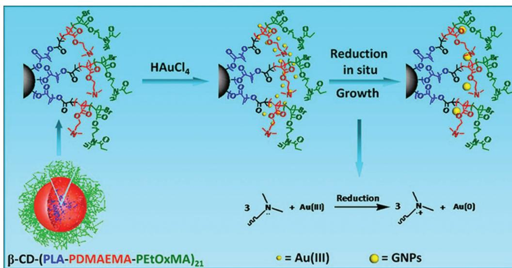
Fig. 19 Schematic representation of using the star-like block copolymer  $\beta\text{-CD}-(\text{PLA-PDMAEMA-PtOxMA})_{21}$  as a unimolecular micelle template for the synthesis and stabilization of gold nanoparticles. Reproduced with permission from Wiley.<sup>201</sup>
