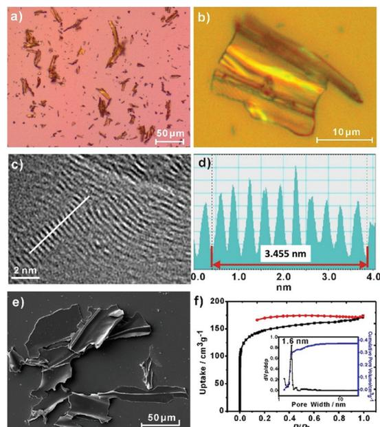
**Fig. 1** 2DPPV: (a, b) optical microscope images; (c) HR-TEM image; (d) the white line trace from (c) shows the resolution of the interlayer distance at about  $\sim 0.35\text{ nm}$ ; (e) SEM image; (f) nitrogen adsorption–desorption isotherms, with the pore size distribution shown in the inset.
