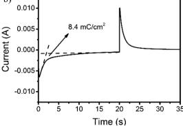
Current consumption upon (a) repeated and (b) enlarged electrochromic switching between 0 and 0.8 V of the 3,6-Cbz-EDOT on the ITO-coated glass plate.
