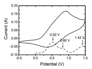
Fig. 3 Cyclic voltammetry (solid line) and differential pulse voltammetry (dotted line) of 3.6-Cbz-EDOT films on an ITO electrode, measured in CH<sub>3</sub>CN with 0.1 M  $(nC_4H_9)_4NPF_6$  at the scan rate of 0.1 V s<sup>-1</sup> under flowing nitrogen.
