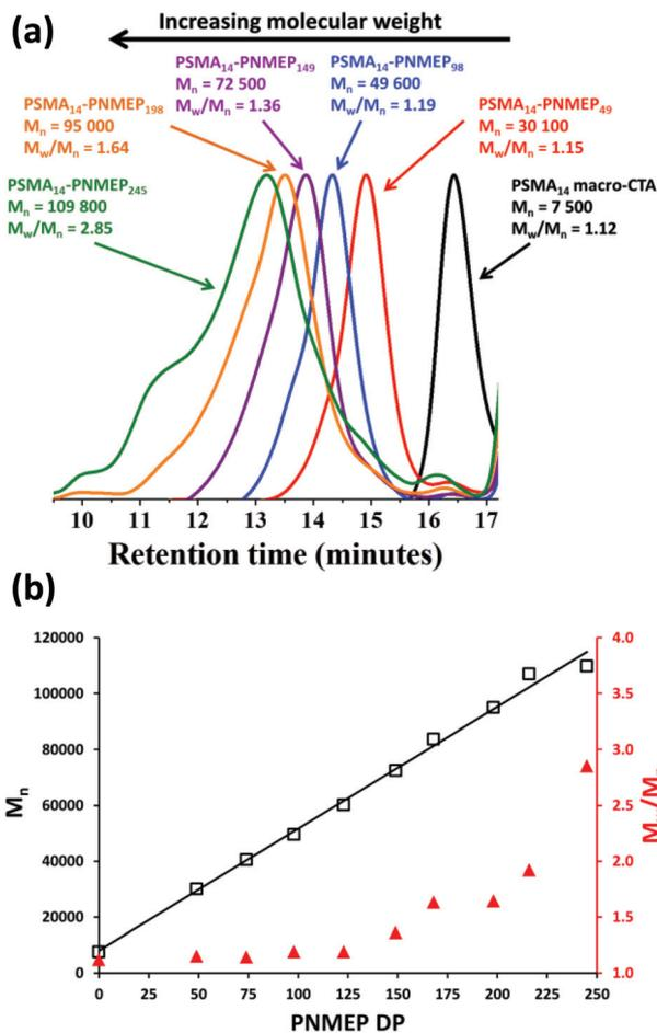
Fig. 2 (a) 3 : 1 Chloroform/methanol GPC curves obtained for PSMA<sub>14</sub>-PNMEP<sub>x</sub> diblock copolymer nanoparticles prepared at 10% w/w solids via RAFT dispersion polymerisation of NMEP at 90 °C. (b) Relationship between target PNMEP DP and GPC  $M_n$  (black squares) and  $M_w/M_n$  (red triangles) for the same series of PSMA<sub>14</sub>-PNMEP<sub>x</sub> diblock copolymer nanoparticles prepared at 10% w/w solids.
