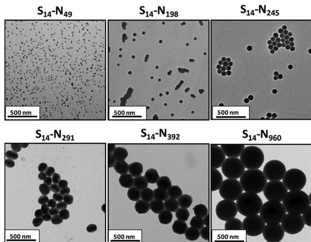
Fig. 4 TEM images obtained for PSMA<sub>14</sub>-PNMEP<sub>x</sub> diblock copolymer nanoparticles prepared at 10% w/w solids in *n*-dodecane showing well-defined spherical nanoparticles (N.B. for brevity 'S' denotes PSMA and 'N' denotes PNMEP).
