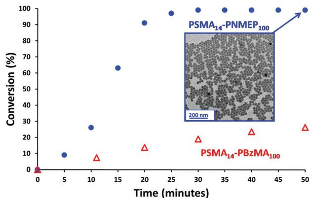
**Fig. 1** Kinetics of the polymerisation of NMEP and BzMA at 90 °C when targeting PSMA<sub>14</sub>-PNMEP<sub>100</sub> (blue circles) and PSMA<sub>14</sub>-PBzMA<sub>100</sub> (red triangles) at 20% w/w solids. Inset: transmission electron microscopy image obtained after 50 min for PSMA<sub>14</sub>-PNMEP<sub>100</sub> showing the formation of near-monodisperse spherical nanoparticles with a mean diameter of 27 nm.
