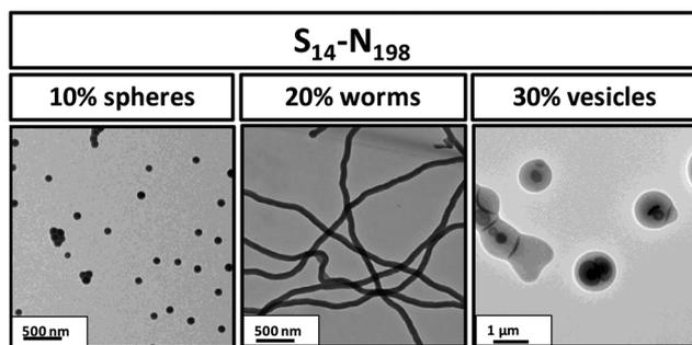
**Fig. 6** TEM images obtained for PSMA<sub>14</sub>-PNMEP<sub>198</sub> diblock copolymer nano-objects prepared at 10, 20 or 30% w/w solids confirming the formation of well-defined spheres, highly anisotropic worms and poly-disperse vesicles, respectively (N.B. for brevity 'S' denotes PSMA and 'N' denotes PNMEP).
