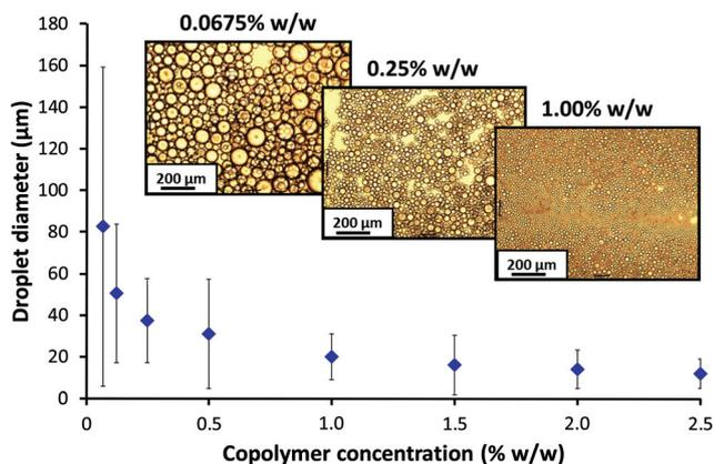
**Fig. 8** Concentration dependence of the mean volume-average droplet diameter (as determined by laser diffraction) for oil-in-water Pickering emulsions prepared at a constant shear rate of 13 200 rpm using PSMA<sub>14</sub>–PNMEP<sub>49</sub> spheres. The error bars shown represent the standard deviation of each mean volume-average droplet diameter, rather than the experimental error. Inset: optical microscopy images of the droplets prepared at 0.0675, 0.25 and 1.00% w/w. Scale bar = 200 µm.
