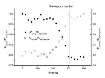
Fig. 3 Comparison of the normalized absorbances of the epoxy and hydroxyl bands during the curing of DG174S3-0.5 formulation at 80 °C.
