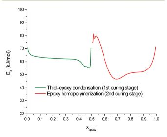
Apparent activation energy of the thiol-epoxy condensation and the excess epoxy homopolymerization during curing of the DG174S3-0.5 formulation, expressed with respect to the epoxy conversion.
