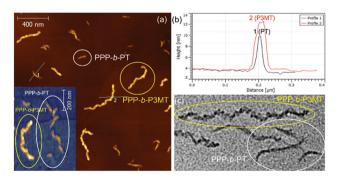
Fig. 4 Comparison between (a) AFM images, (b) height profiles, and (c) TEM images obtained from the mixtures of nanostructures from PPP<sub>70</sub> $b-P3MT_{70}$  ( $M_{\rm p}=18.3{\rm k}$  and PDI = 1.06 of PPP, actual DP of P3MT = 65,  $L_{\rm p}$ = 315 nm,  $L_w/L_n$  = 1.34) and PPP<sub>70</sub>-b-PT<sub>90</sub> ( $M_n$  = 20.5k and PDI = 1.05 of PPP, actual DP of PT = 61,  $L_n$  = 127 nm,  $L_w/L_n$  = 1.17).
