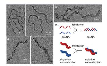
Fig. 3 TEM images of the nanostructures from PPP-b-P3MTs on a Cu/ C TEM grid: (a)  $PPP_{70}$ -b- $P3MT_{50}$ , (b)  $PPP_{70}$ -b- $P3MT_{115}$  and (c)  $PPP_{70}$ -b-P3MT<sub>180</sub>. (d) Schematic comparison between the formation of doublestranded DNA (dsDNA) and multi-line nanocaterpillars.
