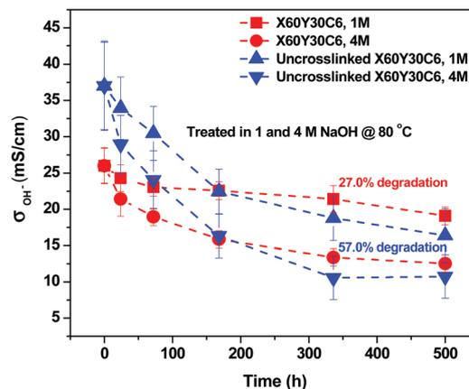
Fig. 8 Chemical stability of the quaternary ammonium cation of X60Y30C6 and uncross-linked X60Y30C6 in 1 M and 4 M NaOH solutions, respectively, at 80 °C, and OH<sup>−</sup> conductivity as a function of duration time measured at 20 °C.
