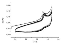
Fig. 9 Repeated cyclic voltammetry curves (10 cycles) of the CpCoCbMA monomer (top) and poly(CpCoCbMA) (bottom) in  $CH_2Cl_2$  with TBAHFP (0.1 M) as an electrolyte. Scan rate was 20 mV s $^{-1}$ .
