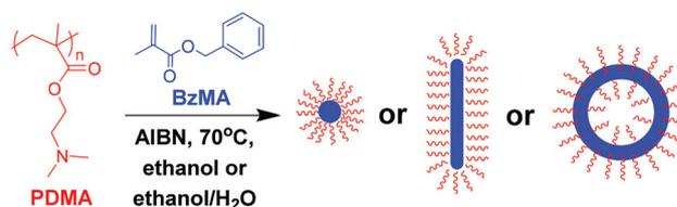
**Scheme 1** Reaction scheme for the synthesis of diblock copolymer nano-objects prepared *via* RAFT alcoholic dispersion polymerization of benzyl methacrylate (BzMA) at 70 °C using a poly(2-(dimethylamino)ethyl methacrylate) (PDMA) chain transfer agent. AIBN initiator was used at a [PDMA]/[AIBN] molar ratio of 5. The final diblock copolymer morphology can be spheres, worms or vesicles, depending on the precise diblock copolymer composition.
