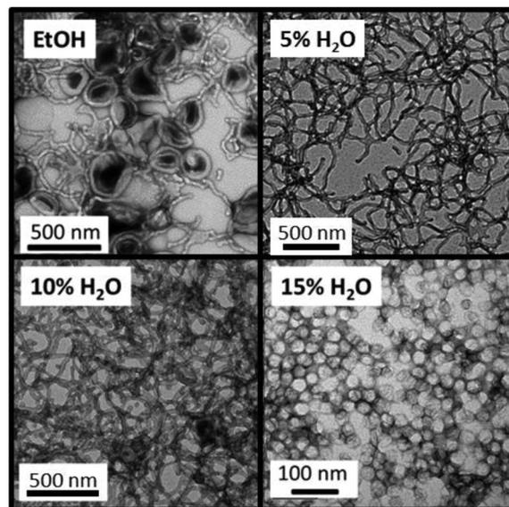
**Fig. 6** TEM images of PDMA<sub>43</sub>-PBzMA<sub>120</sub> nano objects prepared via RAFT dispersion polymerization of BzMA at 15% w/w in anhydrous ethanol or ethanol/water at 70 °C using AIBN initiator ([PDMA<sub>43</sub>]/[AIBN] = 5). The solvent composition is indicated in each case and the morphology varies from a mixed vesicle/worm phase to pure worms to mixed worms/spheres and finally pure spheres as the water content of the continuous phase is increased from 0% to 15% w/w.
