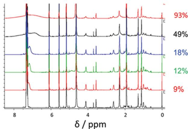
**Fig. 2**  $^1\text{H}$  NMR spectra recorded during the RAFT dispersion polymerization of BzMA at  $70^\circ\text{C}$  in  $d_6$ -ethanol targeting a final diblock composition of PDMA<sub>43</sub>-PBzMA<sub>500</sub>. Monomer conversions were calculated by comparing the integrals of the vinyl monomer to the  $t = 0$  spectrum using TMS as the internal standard.
