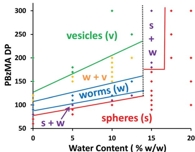
**Fig. 5** Phase diagram showing the morphology obtained for PDMA<sub>43</sub>-PBzMA<sub>x</sub> diblock copolymers synthesized via RAFT dispersion polymerization of BzMA at 70 °C in either anhydrous ethanol or various ethanol/water mixtures at 15% w/w solids. Conditions: [PDMA<sub>43</sub>]/[AIBN] = 5.0.
