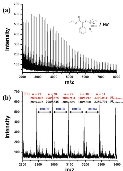
Fig. 6 (a) MALDI-TOF mass spectrometry results in the round mode of PMMA ( $M_{n,\text{GPC}} = 13\,800 \text{ g mol}^{-1}$ ,  $M_w/M_n = 1.53$ ) obtained by metal-free ATRP of MMA with fluorescein (FL) as an organic photocatalyst. (b) Enlargement of the MALDI-TOF-MS of PMMA from  $m/z$  2800 to 3400.
