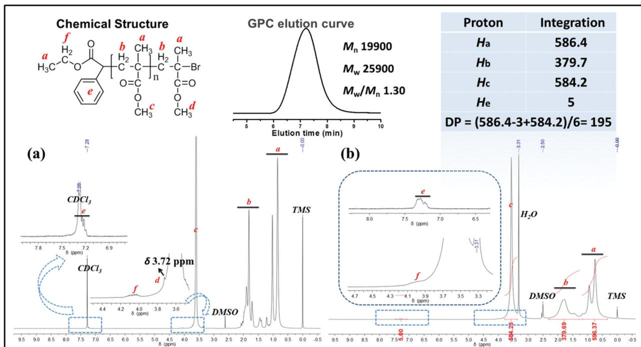
Fig. 4 <sup>1</sup>H NMR spectra of PMMA in CDCl<sub>3</sub> (a) and DMSO-*d*<sub>6</sub> (b), obtained by photoinduced metal-free PET-ATRP of MMA under conditions of  $[MMA]_0 : [EBPA]_0 : [FL]_0 : [TEA]_0 = 200 : 1 : 0.3 : 9$  in 2.0 mL of DMSO for 5 h.  $M_{n,GPC} = 19\,900$  g mol<sup>-1</sup>,  $M_w/M_n = 1.30$ ,  $M_n,^1H\ NMR = 19\,800$  g mol<sup>-1</sup>.
