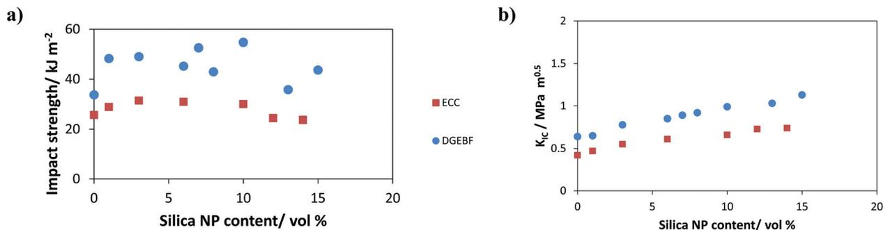
Fig. 10 Toughening effects of SNPs on epoxy thermosets.
