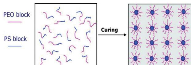
Fig. 14 Reaction-induced microphase separation in BC-toughened thermosets. Reprinted with permission from *Macromolecules*.<sup>109</sup> Copyright 2006 American Chemical Society.
