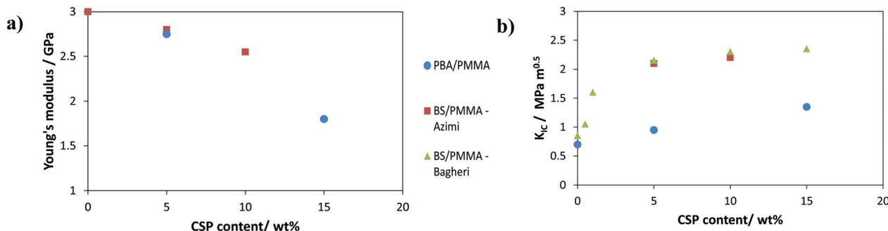
Fig. 13 Effect of CSPs in DGEBA epoxy resins on Young's modulus (a) and fracture toughness (b). Note: Bagheri *et al.* provide values for toughness of BS/PMMA CSPs but do not give values for modulus.<sup>77</sup>
