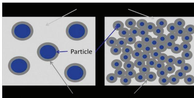
Fig. 9 Schematic comparison of interfacial polymer in conventional composites with micron-sized filler (left) and in nanocomposites (right).
