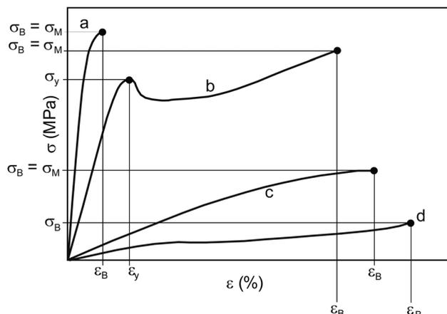
Fig. 1 Exemplary stress–strain curves for various polymers: brittle materials (a), tough materials with yield point (b), tough materials without yield point (c) and elastomers (d).<sup>7</sup>
