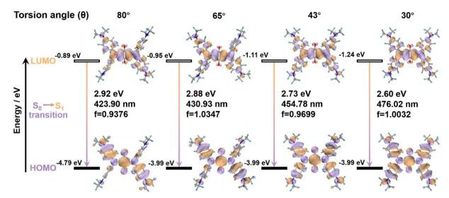
Fig. 4 Energy diagrams and the frontier orbital contribution of SQ-NMe<sub>2</sub> in a fixed conformation based on gradually decreased torsion angels  $(\theta)$  between the central four-membered ring and diphenylamine rotors, together with their lowest-energy transitions estimated by theoretical calculations.
