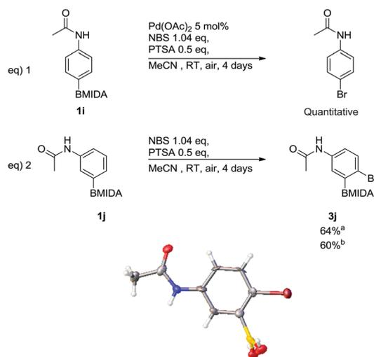
Scheme 5 Attempted bromination *via* *ortho*-selective C–H activation, including X-ray structure of 3j' (MIDA protection was cleaved in crystallisation process). <sup>a</sup> With 5 mol% Pd(OAc)<sub>2</sub>, <sup>b</sup> without Pd(OAc)<sub>2</sub>.
