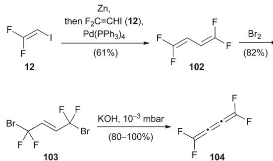
**Scheme 26** Negishi cross-coupling with 1,1-difluoro-2-iodoethene (**12**) and formation of tetrafluorobutatriene (**104**).
