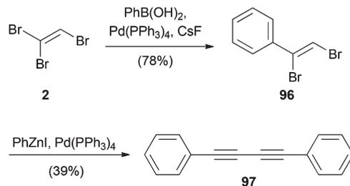
**Scheme 24** Suzuki–Miyaura cross-coupling with TBE (**2**) and subsequent homocoupling under Negishi cross-coupling conditions.
