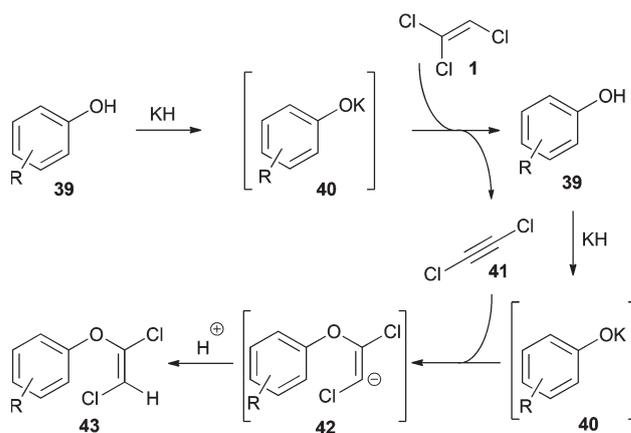
Scheme 8 Mechanism of the elimination–addition reaction of 1 using potassium phenolates 40.
