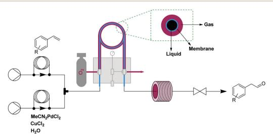
Fig. 3 Transformer 2 – oxidation: using oxygen, delivered by a tube-in-tube reactor, showcased with the transformation of styrenes into aldehydes.<sup>12</sup>
