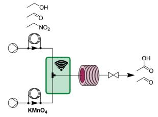
Fig. 4 Transformer 3 – oxidation: using a liquid phase oxidant and an ultrasonic bath (green box) to avoid aggregation of precipitants resulting from oxidation byproducts.  $^{13}$
