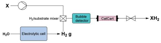
Fig. 6 Transformer 5 – reduction: using in situ generated hydrogen by electrolysis of water, which under pressure creates a saturated solution that passes through a packed bed reactor containing the catalyst. 16
