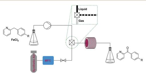
Fig. 2 Transformer 1 – oxidation: using oxygen, creating a biphasic gas-liquid system using a T-mixer, exemplified by a benzylic oxidation procedure with iron(III) chloride.10
