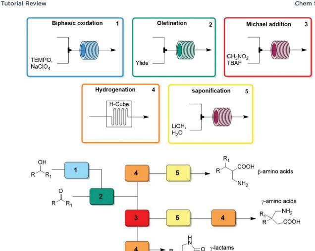
Fig. 28 CAS 5 –  $\beta$ -amino acids,  $\gamma$ -lactams,  $\gamma$ -amino acids: a divergent CAS synthesizes libraries of three different functional cores. Levels of control: starting material choice, reagent choice, and order of modules.
