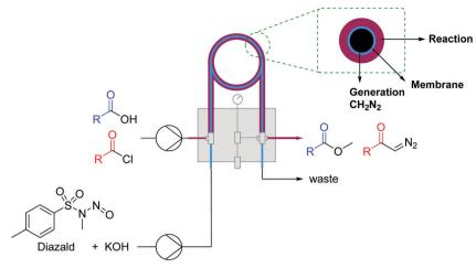
Fig. 18 Generator 6 – dizaomethane: generation of diazomethane and reactions thereof in a tube-in-tube reactor.<sup>33</sup>
