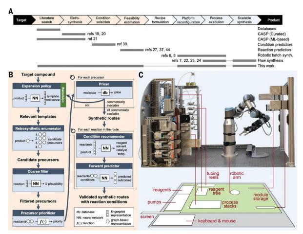
Fig. 30 Auto-CAS 1 – linear syntheses: an automated, robotic platform for the flow synthesis of organic compounds informed by AI planning. 49 From Science, 2019, 365, eaax1566. Reprinted with permission from AAAS.
