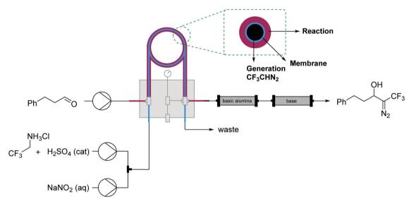
Fig. 19 Generator 7 – alkyl diazo compounds: generation of fluorinated diazo compounds and use *via* a tube-in-tube reactor. The generator is coupled with a packed-bed reactor to catalyze an aldol coupling of the formed diazo intermediate.<sup>34</sup>
