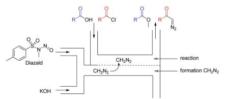
Fig. 17 Generator 5 – diazomethane: dual stream in situ generation and reaction of diazomethane via a membrane reactor. 32
