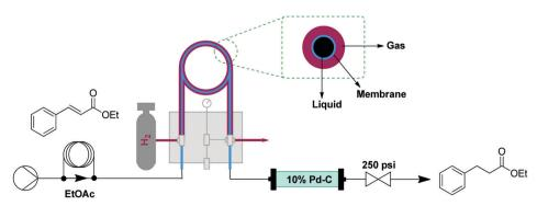
Fig. 5 Transformer 4 – reduction: using hydrogen gas delivered by a tube in tube reactor and catalyst *via* a packed bed reactor (where the reduction takes place). <sup>15</sup>
