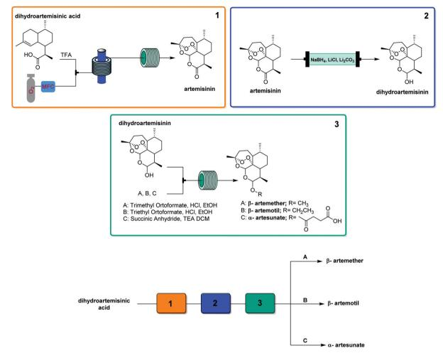
Fig. 24 CAS 1 – artemisinin derivatives: a modular system for the synthesis of antimalarial APIs. Level of control: starting material choice.
