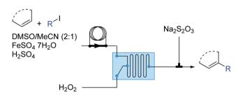
Fig. 16 Generator 4 – alkyl radicals: two-step process for formation of alkyl radicals, with selective trapping with an *in situ* alkene.<sup>30</sup>
