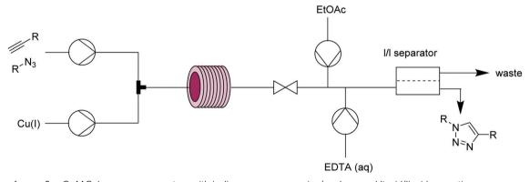
Fig. 10 Transformer 9 – CuAAC: homogeneous system with in-line copper scavenging/work-up and liquid/liquid separation.
