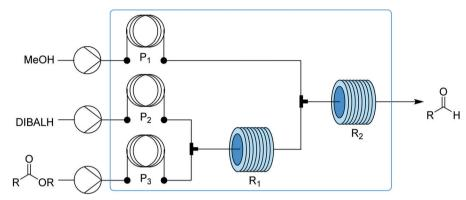
Fig. 7 Transformer 6 – reduction: controlled homogeneous partial reduction of esters to aldehydes using hydride.<sup>17</sup> Blue box corresponds to the chilled section of the transformer
