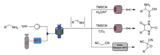
Fig. 25 CAS 2 - divergence from imines: generator 10 (singlet oxygen) is coupled with one of three different modules to give three classes of compounds. Levels of control: starting material choice and order of modules
