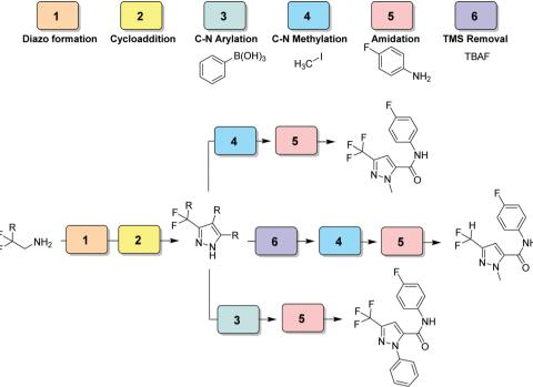
Fig. 29 CAS 6 – pyrazole library: a six module divergent CAS exhibits controlled functionalization of multiple positions of the formed pyrazole moiety. 48
