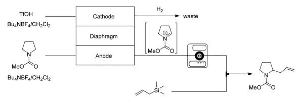
Fig. 13 Generator 1 – cations: electrolytic generation of iminium ions, capable of inline monitoring, delivered to a stream containing the nucleophile.<sup>27</sup>
