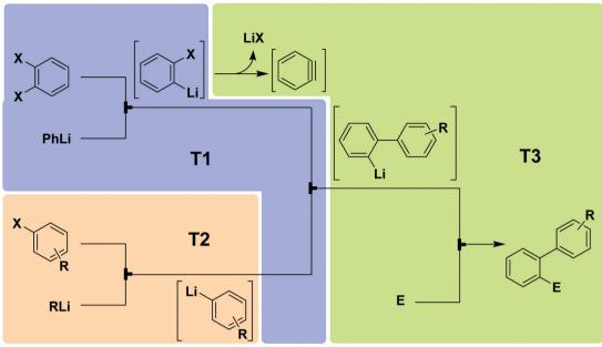
Fig. 14 Generator 2 – benzyne: fully adjustable three-component system for generating and utilizing benzyne with different nucleophiles and electrophiles.<sup>28</sup> The three temperature zones are shown with colored boxes.
