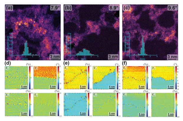
Fig. 4 Dislocation density analysis at stitched grain boundaries. (a–c) Atomic-resolution HAADF-STEM images of the three grain boundaries. Insets show the distributions for distances between the dislocation cores for each boundary. (d–f) Strain maps for each boundary, calculated with geometric phase analysis: shear strain ( $\varepsilon_{xy}$ ), rotation ( $\gamma_{xy}$ ),  $\varepsilon_{xx}$  and  $\varepsilon_{yy}$  strain field. The features at the edges of the images are boundary artifacts.
