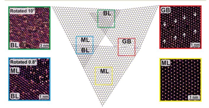
Fig. 1 A schematic representation of the formation of stitched grain boundary (GB) structures between two monolayer (ML) grains and bilayer (BL) stacking in overlap areas. HAADF-STEM images of MoS<sub>2</sub> GB and BL stacking of MoS<sub>2</sub> are shown in the colored frames.
