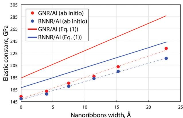
Fig. 2 Dependence of the *ab initio* calculated (filled circles) and estimated from eqn (1) (solid lines) uniaxial elastic constant  $C$  of the BN/graphene nanoribbons/Al-composite on the width of the ribbons embedded into Al. The data for graphene and BN nanoribbons are depicted by red and blue color, respectively. By zero width the values of the elastic constant of monoatomic BN/carbon chains are presented.
