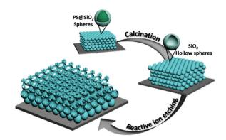
Fig. 1 Schematic illustration of the fabrication process for producing 3D hierarchical nanostructures by direct etching of hollow SiO<sub>2</sub> sphere colloidal crystals via reactive ion etching.
