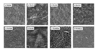
Scanning electron microscopy (SEM) of PMMA-supported diacetylene films. The films comprised the indicated derivatives and the TRCDA (1) monomer at 1:1 mole ratio. Scale bars correspond to 10 µm.
