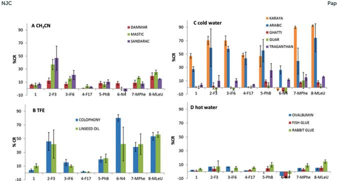
Fig. 4 Colorimetric responses of PMMA-supported PDA films comprising different derivatives to paint substances. %CR values after subtraction of the buffer divided according to the solvent used for dissolving the material. (A) Materials dissolved in acetonitrile (terpenic compounds); (B) materials dissolved in trifluoroethanol TFE (triglycerides, colophony); (C) materials dissolved in cold water (gums); (D) materials dissolved in hot water (proteinaceous materials).
