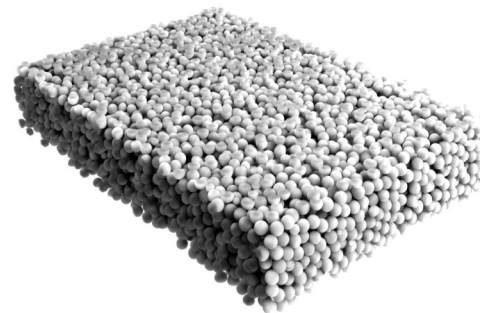
Fig. 6 Reconstructed bed of 2.6 \mu\text{m} spherical core-shell particles packed into a 100 \mu\text{m} inner-diameter cylindrical fused-silica capillary. The reconstruction covers a capillary segment of 100 \mu\text{m} (entire capillary diameter) \times 58 \mu\text{m} (along the column axis) \times 15 \mu\text{m} . The imaging of the packing microstructure is based on confocal laser scanning microscopy, realized by adapting a refractive index matching approach. 108
