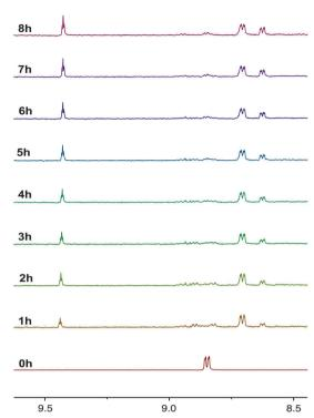
Fig. 5 <sup>1</sup>H NMR progression of the photolysis of 2a in deuterated acetonitrile solutions. The photolysis was performed by irradiating the sample at 365 nm over a period of 8 h.
