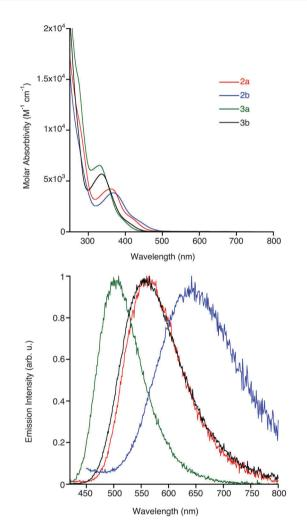
Fig. 3 Experimental absorption (top) and emission profiles (bottom) of the complexes from dilute dichloromethane solutions (ca.  $10^{-5}$  M) at room temperature. The emission profiles were obtained by exciting the complexes to their lowest energy  $\lambda_{abs}$ . The same colour coding (inset) is used between the absorption and emission profiles.
