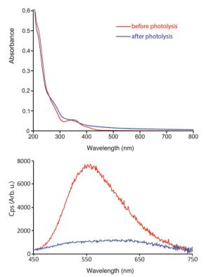
Fig. 8 Experimental absorption (top) and emission (bottom) profiles of 2a from dilute acetonitrile solutions (ca.  $10^{-5}$  M) at room temperature before and after exhaustive photolysis. The emission profiles were obtained by exciting the complex at 350 nm. The same colour coding is used between the absorption and emission profiles.
