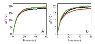
Fig. 3 (A) Thermograms ( $\Delta T$  vs. t) for Type II surfaces, obtained by irradiation at 800 nm with a 200 mW laser source on a 1 cm diameter spot (irradiance = 0.25 W cm<sup>-2</sup>). The three profiles refer to three different slides from the same preparation. (B) Same as A, for Type III surfaces. The profiles with the same colour are from the same slide, before (A) and after (B) coating with  $[Cu_2L]^{4+}$ .
