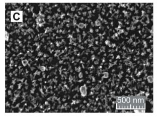
Fig. 2 (A) Extinction spectra of Type II surface (blue color) and of Type III surface obtained from it (red color); (B) TEM image of a GNS used for coating (see ESI,† Fig. S3 for complete image); (C) SEM image of a Type II surface (particular; see ESI,† Fig. S1 for full image and additional images).
