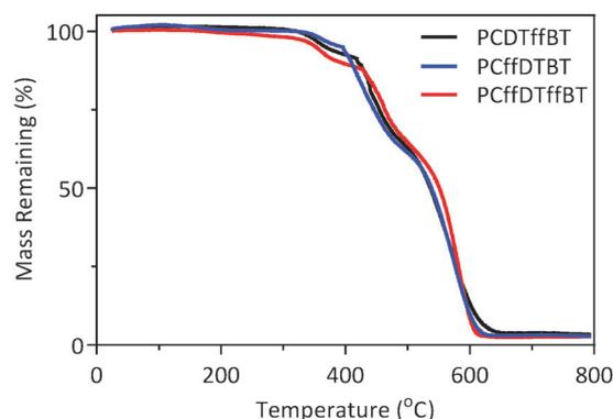
Fig. 5 Thermogravimetric analysis of **PCDTffBT**, **PCffDTBT** and **PCffDTffBT** with a heating rate of 10 °C min<sup>-1</sup> under an inert nitrogen atmosphere.
