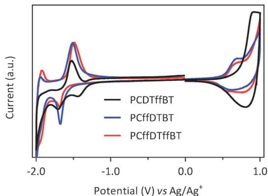
Fig. 4 Cyclic voltammograms of **PCDTffBT**, **PCffDTBT** and **PCffDTffBT** on platinum disc electrodes (area 0.031 cm<sup>2</sup>) at a scan rate of 100 mV s<sup>-1</sup> in acetonitrile/tetrabutyl ammonium perchlorate (0.1 mol dm<sup>-3</sup>).
