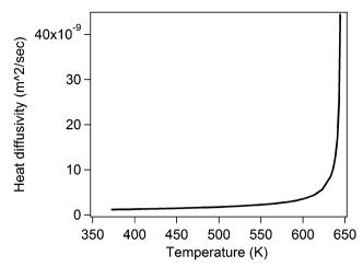
**Fig. 8** This plot shows the value of the thermal diffusivity as a function of temperature. The value of the diffusivity becomes very large as the critical temperature of water is reached. The different constants used for the diffusivity of water are obtained from the engineering tables.<sup>27</sup>
