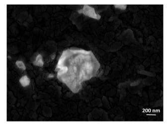
Fig. 9 SEM image of the post reaction SOM 1.
