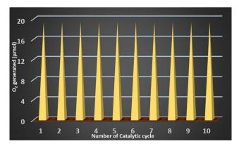
Fig. 10 Catalytic recyclability of the composite catalyst SOM 1.
