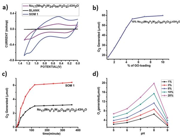
Fig. 5 (a) Cyclic voltammogram of the water oxidation study by the POM  $Na_{17}[Mn_6P_3W_{24}O_{94}(H_2O)_2]\cdot 43H_2O$  and SOM **1**. (b) Extent of oxygen liberated with variation in graphene oxide-loading with  $Na_{17}[Mn_6P_3W_24O_{94}(H_2O)_2]\cdot 43H_2O$  concentration kept constant. (c) Comparative oxygen evolution by the POM  $Na_{17}[Mn_6P_3W_{24}O_{94}(H_2O)_2]\cdot 43H_2O$  only and SOM **1**. (d) Variation of oxygen yield with pH.
