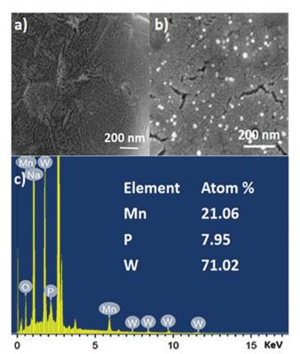
Fig. 3 SEM images of (a) graphene oxide surface. (b) SOM 1, defined by aggregate nanospherical POMs immobilized on the graphene oxide layers. (c) EDX spectrum of SOM 1.
