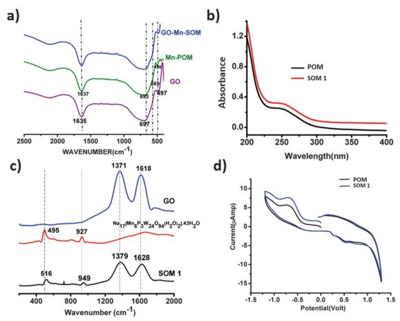
Fig. 4 (a) HATR-IR spectroscopy of the POM constituent, GO, and SOM 1. (b) UV-VIS spectroscopy of the POM constituent of SOM 1 and SOM 1. (c) Raman spectra of the POM unit  $Na_{17}[Mn_6P_3W_{24}O_{94}(H_2O)_2]$ -43H<sub>2</sub>O, graphene oxide and SOM **1**. (d) Cyclic voltammogram of SOM **1** and the POM constituent of SOM 1.
