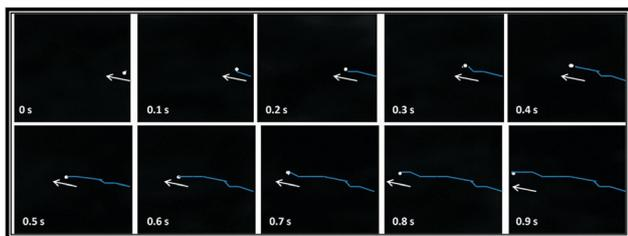
Fig. 4 Time lapse images of moving SOM in  $0.014 \text{ mol L}^{-1}$  sodium dithionite. The direction of motion is shown by the arrow and the blue lines indicate the trace lines.
