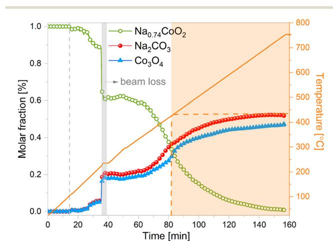
Fig. 6 Evolution of temperature and sample weight percent during NaCoO<sub>2</sub> carbonation reaction according to results from Rietveld analysis.
