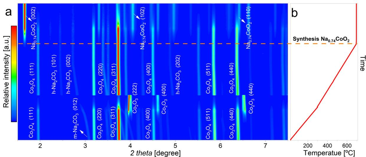
Fig. 3 a) Contour plot of the XRD patterns collected during the synthesis of  $\text{NaCoO}_2$ , starting from  $m\text{-Na}_2\text{CO}_3$  and  $\text{Co}_3\text{O}_4$  powders, b) temperature evolution during the solid-state synthesis of  $\text{NaCoO}_2$ .
