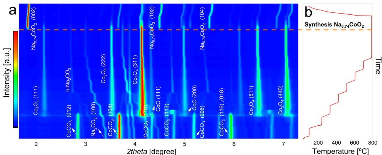
Fig. 1 a) Contour plot of the XRD patterns collected during the synthesis of NaCoO<sub>2</sub> from CoCO<sub>3</sub> and *m*-Na<sub>2</sub>CO<sub>3</sub> precursors, b) evolution of the temperature and time during the synthesis process.
