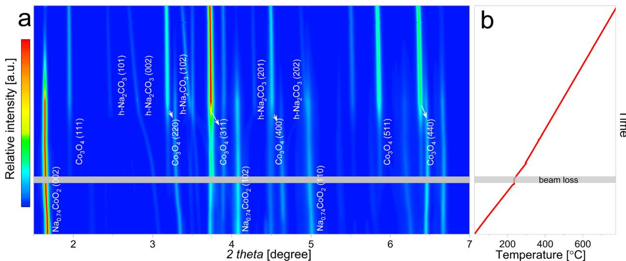
Fig. 5 a) Contour plot displaying XRD data corresponding to NaCoO<sub>2</sub> dynamic heating under CO<sub>2</sub> gas flow until 750 °C, b) temperature evolution during NaCoO<sub>2</sub> carbonation process.
