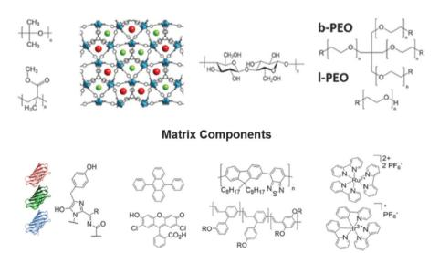
Fig. 2 Upper part – exemplary of the components used for the matrix – *i.e.*, cross-linked polymers (left), MOF (central left), cellulose (central right), and non-cross-linked branched (b-PEO) and linear (l-PEO) polyethyleneoxide derivatives (right). Lower part – exemplary of the luminescent materials – *i.e.*, fluorescent proteins (left), small-molecules (central left), polymers (central right), and coordination complexes (right).
