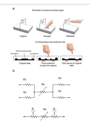
Fig. 2 Flexible microfluidic pressure sensor. (a) Working principle as a micropump system when the load is applied and removed, respectively. (b) Principle of operation illustrated using an electrical circuitry analogy
