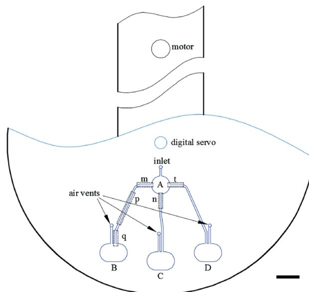
**Fig. 8** Schematic of a design that uses a 2-DoF centrifugal microfluidic platform to achieve targeted flow switching. The flow switching device is designed to enable fluid to be pumped from an original chamber (A) to one of the target chambers (B, C or D) on demand. All target chambers are equipped with air vents. When channels m, n or t are collinear with the centre of the motor, the liquid will be pumped into chambers B, C and D respectively. The scale bar is 5 mm.
