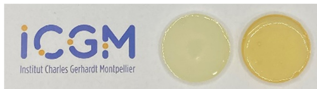
Fig. 1 Picture of MDI-based thermoset (left) and BGI-based thermoset (right).
