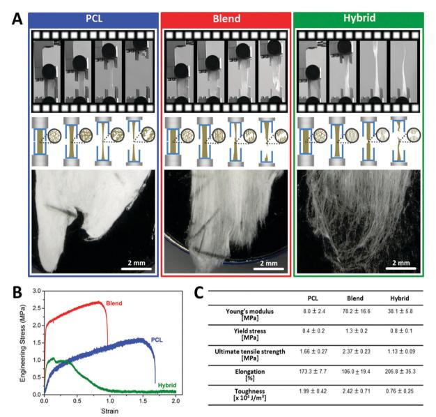
Fig. 3 Mechanical properties of electrospun PCL, blend and hybrid fiber mats. (A) Visualization of the different failure modes based on acquired timelapsed serial images upon tensile loading and representative optical micrographs of the fracture fiber surfaces after mechanical testing. (B) Typical engineering stress-strain curves for each type of fiber mats. (C) Mechanical parameters calculated from the engineering stress-strain curves.
