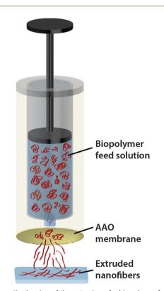
Fig. 1 Schematic drawing of the extrusion of a biopolymer feed solution through a nanoporous AAO membrane. Extruded nanofibers are collected on a glass slide for further analysis.
