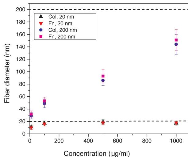
**Fig. 4** Dependence of the nanofiber diameter on the AAO pore diameter and the protein concentration measured for collagen and fibronectin. The dashed lines indicate the two different nanopore diameters of 20 nm and 200 nm, which were used for the extrusion experiments with varying concentration of the protein solution. With increasing protein concentration the nanofiber diameter approaches the size of the AAO nanopores.
