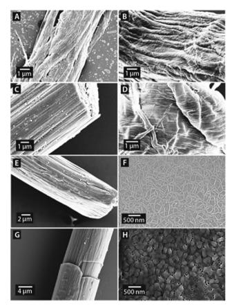
**Fig. 3** (A–F) SEM images of nanofibrous ECM protein structures, which were extruded with  $c=10~\mu g~ml^{-1}$  and  $d_{AAO}=200~nm$  and deposited onto glass slides with either PLL or PFA coating: (A) collagen on PLL, (B) fibronectin on PLL, (C) fibrinogen on PFA, (D) elastin on PLL, (E) laminin on PFA, (F) collagen on PLL, (G) fibronectin extruded onto PFA coated glass, (H) emerging collagen nanofibers from AAO nanopores after extrusion ( $c=10~\mu g~ml^{-1}$ ,  $d_{AAO}=70~nm$ , PFA).
