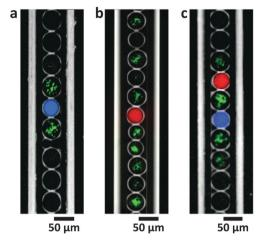
Fig. 3 Inducer reservoir droplets. Fluorescence microscopy images of bacterial AND gate droplets in the presence of (a) an AHL reservoir droplet (blue, [AHL] = 200 nM) with IPTG globally, (b) an IPTG reservoir droplet (red, [IPTG] = 10 mM) and AHL globally. (c) Gene expression of bacterial AND gate operated localized by a reservoir droplet of AHL (blue, [AHL] = 200 nM) and in the vicinity of IPTG reservoir droplet (red, [IPTG] = 10 mM).
