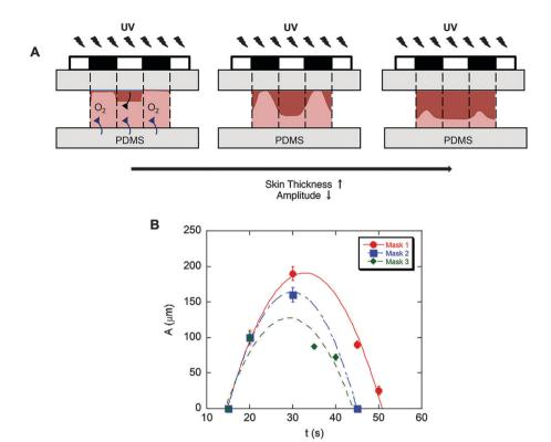
Fig. 3 Evolution of patterned substrates with time. (A) The competition between radical polymerization and diffusion of radical scavenger  $O_2$ . (B) Pattern amplitude with UV exposure time for each mask indicates biphasic behavior. Pattern amplitude (height) was measured using SEM images. The error bars denote standard deviation (3 images for each sample, n = 3 samples for each condition).
