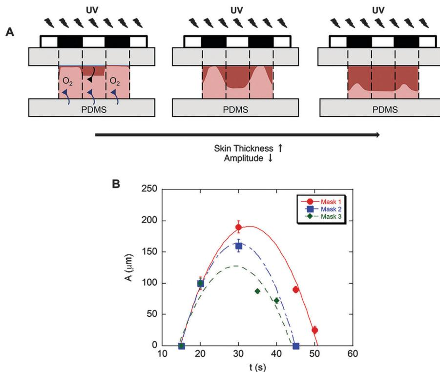
Fig. 3 Evolution of patterned substrates with time. (A) The competition between radical polymerization and diffusion of radical scavenger O<sub>2</sub>. (B) Pattern amplitude with UV exposure time for each mask indicates biphasic behavior. Pattern amplitude (height) was measured using SEM images. The error bars denote standard deviation (3 images for each sample,  $n = 3$  samples for each condition).
