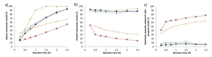
Fig. 1 Xylose hydrogenation reactions with Ru/C (black filled circles), Ru0.6/USY9 (red squares), Ru0.6/USY3 (green triangles), Ru/C + HCl (orange crosses) and HCl treated Ru/C (blue open circles): (a) xylose conversion, (b) pentitol selectivity and (c) selectivity towards undesired side-products (xylose dehydration products and humins).
