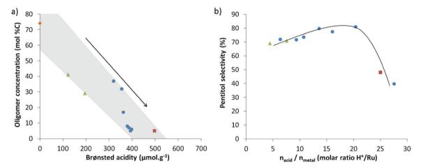
Fig. 2 (a) Influence of the Brønsted acidity on the XO conversion and (b) impact of the molar acid/metal ratio on the pentitol selectivity (which is defined as  $(Y_{pentitol})/(Y_{pentitol} + Y_{degradation products} + Y_{humins}) \times 100$ ): USY9 catalysts (filled blue circles), highly acidic USY19 (red square), low acid USY zeolites (green triangles) and Ru/C (orange rhombus).
