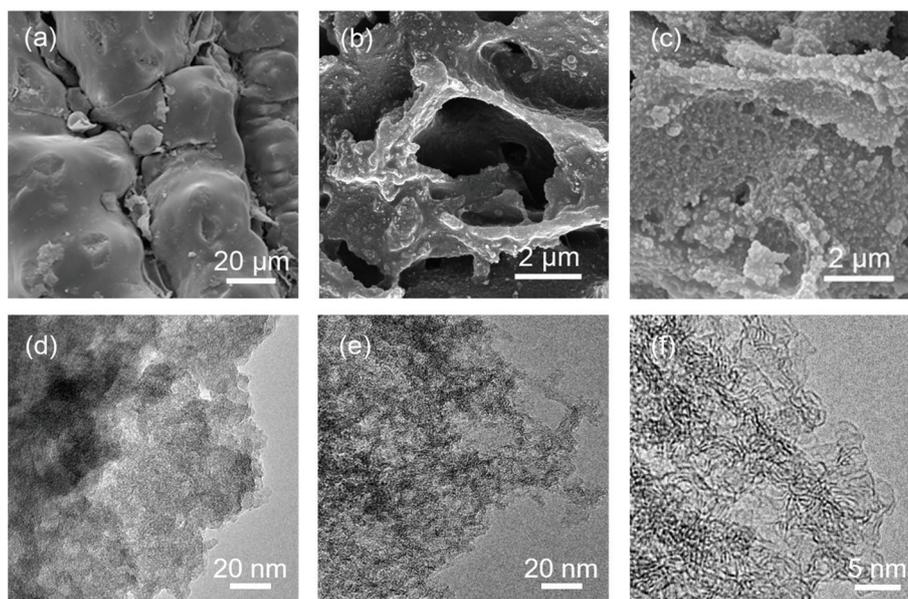
**Fig. 1** Morphology of rice husk derived carbon: SEM images of (a) RHC-SiO<sub>2</sub>, (b) RHC, and (c) RHC-HT. TEM images of (d) RHC-SiO<sub>2</sub> and (e) RHC. (f) High-resolution TEM image of RHC.
