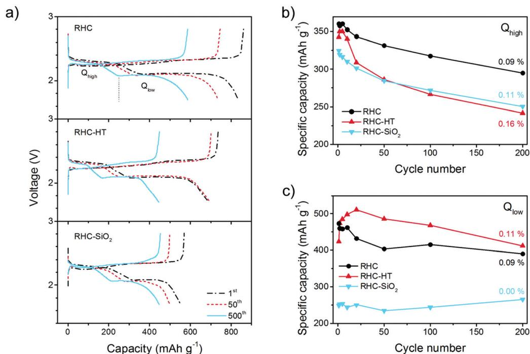
Fig. 7 (a) Galvanostatic charge–discharge profiles of RHC-HT, RHC-SiO<sub>2</sub>, and RHC at current density of 0.5 C. Capacity retention of different voltage plateaus of RHC-HT, RHC-SiO<sub>2</sub>, and RHC: (b) high plateau (2.3–2.4 V,  $Q_{\text{high}}$ ) and (c) low plateau (2.0–2.1 V,  $Q_{\text{low}}$ ).
