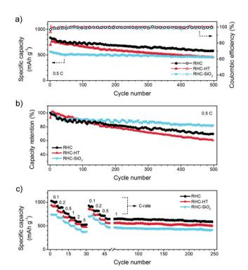
**Fig. 6** Li–S battery performance of RHC-HT, RHC-SiO<sub>2</sub>, and RHC: (a) cycling performance and (b) corresponding capacity retention at a current density of 0.5 C (1C = 1672 mA h g $^{-1}$ ). The open and solid dots in (a) indicate the charge and discharge capacity, respectively. (c) Rate performance. After the rate test, there is a long-term cycling at the current density of 1.0 C.
