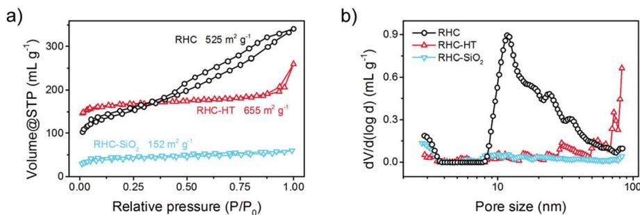
Fig. 3 (a)  $N_2$  isothermal sorption and (b) corresponding pore size distribution based on density functional size theory of RHC-HT, RHC-SiO<sub>2</sub>, and RHC.
