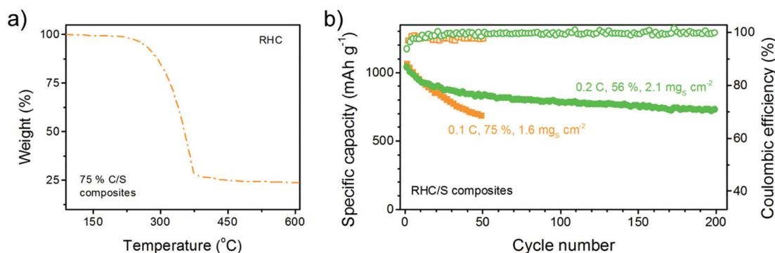
Fig. 11 (a) TG curve of 75% C/S composites and (b) cycling performance of high-sulphur-loading batteries with 56% RHC/S composites at  $2.1 \text{ mg}_s \text{ cm}^{-2}$  or 75% RHC/S composites at  $1.6 \text{ mg}_s \text{ cm}^{-2}$ .
