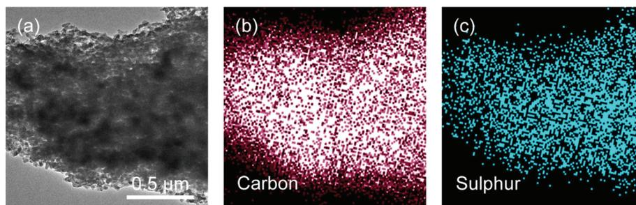
Fig. 4 (a) TEM image and corresponding EDS mapping of (b) carbon and (c) sulphur of 56% RHC/S.
