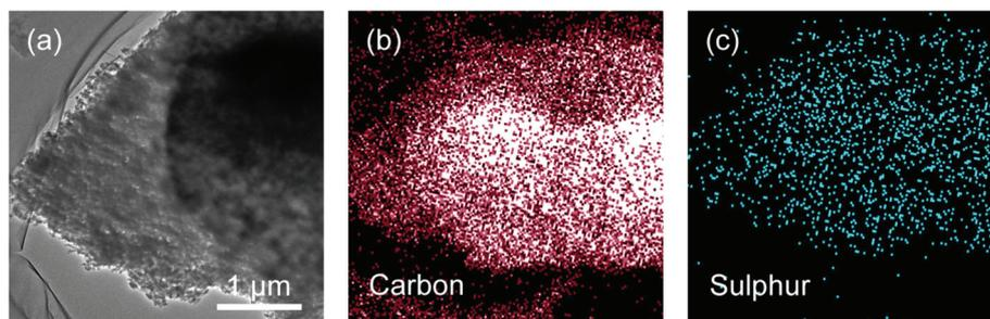
Fig. 10 (a) TEM image and corresponding EDS mapping of (b) carbon and (c) sulphur of 75% RHC/S.
