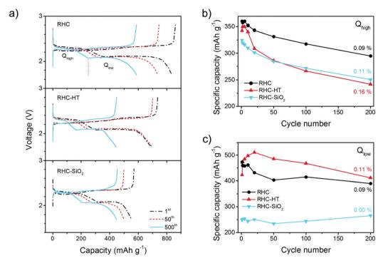
Fig. 7 (a) Galvanostatic charge-discharge profiles of RHC-HT, RHC-SiO<sub>2</sub>, and RHC at current density of 0.5 C. Capacity retention of different voltage plateaus of RHC-HT, RHC-SiO<sub>2</sub>, and RHC: (b) high plateau (2.3–2.4 V,  $Q_{high}$ ) and (c) low plateau (2.0–2.1 V,  $Q_{low}$ ).
