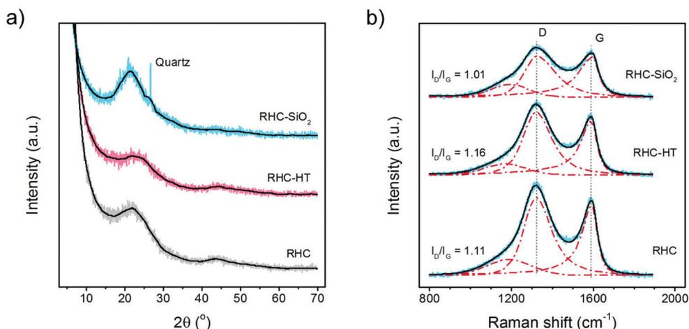
**Fig. 2** (a) XRD patterns and (b) Raman spectra of RHC-HT, RHC-SiO<sub>2</sub>, and RHC.
