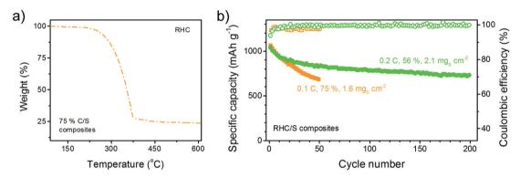
Fig. 11 (a) TG curve of 75% C/S composites and (b) cycling performance of high-sulphur-loading batteries with 56% RHC/S composites at  $2.1 \text{ mg}_{\text{S}} \text{ cm}^{-2} \text{ or } 75\% \text{ RHC/S} \text{ composites at } 1.6 \text{ mg}_{\text{S}} \text{ cm}^{-2}$
