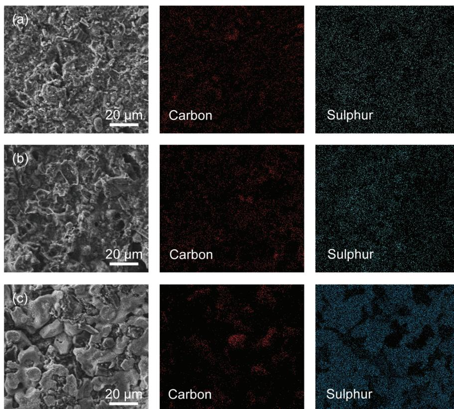
Fig. 9 SEM images and corresponding EDS mapping of carbon and sulphur of cycled C/S electrodes: (a) RHC, (b) RHC-SiO<sub>2</sub>, and (c) RHC-HT.
