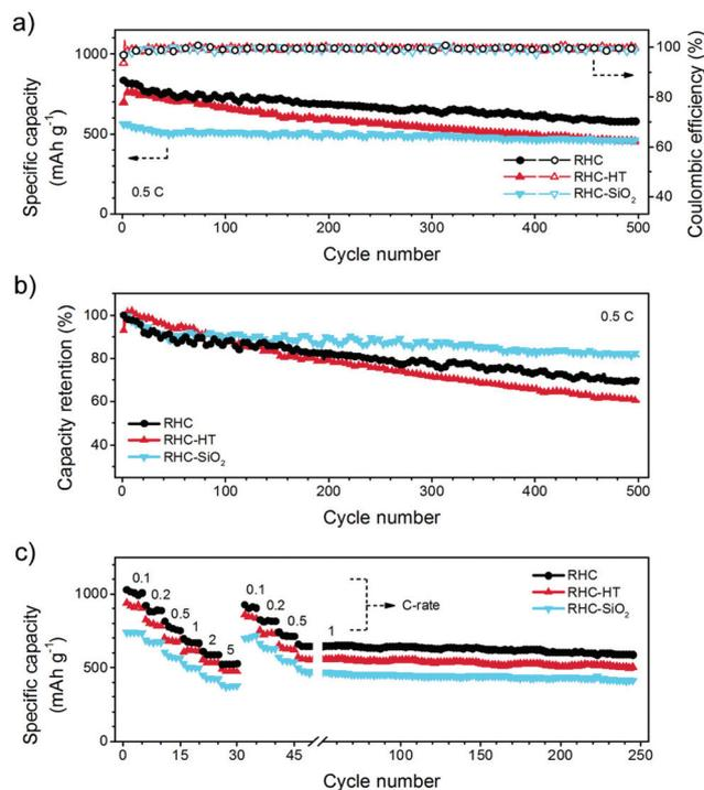
Fig. 6 Li-S battery performance of RHC-HT, RHC-SiO<sub>2</sub>, and RHC: (a) cycling performance and (b) corresponding capacity retention at a current density of 0.5 C (1C = 1672 mA h g<sup>-1</sup>). The open and solid dots in (a) indicate the charge and discharge capacity, respectively. (c) Rate performance. After the rate test, there is a long-term cycling at the current density of 1.0 C.
