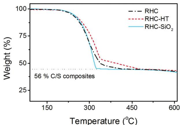
Fig. 5 Thermogravimetric (TG) analysis on C/S composites of RHC-HT, RHC-SiO<sub>2</sub>, and RHC.
