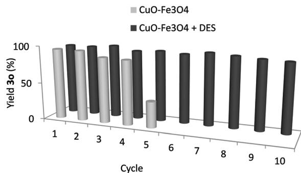
Fig. 3 Recycling of the CuO-Fe<sub>3</sub>O<sub>4</sub> catalyst and CuO-Fe<sub>3</sub>O<sub>4</sub> + DES.
