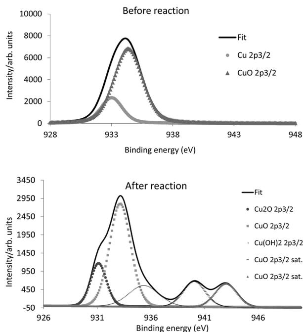
Fig. 5 XPS of fresh and recycled copper catalyst.
