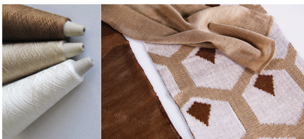
Fig. 6 Yarns and final knitted garments made of fibers spun from bleached pulp (white), cardboard (beige), and pulp with additional lignin added (brown).
