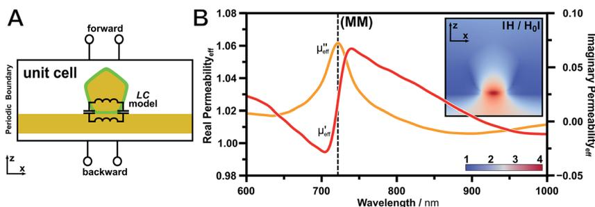
Fig. 5 Effective magnetic properties of film-coupled nanorods. (A) Schematic representation of the *S*-parameter retrieval method and analogy to the inductor–capacitor (*LC*) model. The unit cell is treated as an effective medium, since only the *S*-parameters are evaluated in the forward and backward direction. (B) Calculated magnetic permeability for the film-coupled nanorod revealing the presence of a magnetic resonance and related magnetic field (inset).
