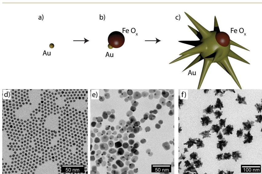
**Fig. 1** Scheme of the synthesis of Janus magnetic nanostars through consecutive seed-and-growth-steps. (a) Oleylamine synthesis of Au nanoparticles. (b) Growth of an iron oxide nanoparticle through the decomposition of  $\text{Fe}(\text{CO})_5$  and subsequent oxidation. (c) Growth of an Au nanostar coated with PVP using the NDs as seeds (d–f) TEM images of different nanoparticles corresponding to the scheme above: (d) Au NPs, (e) NDs, (f) JMNSs.
