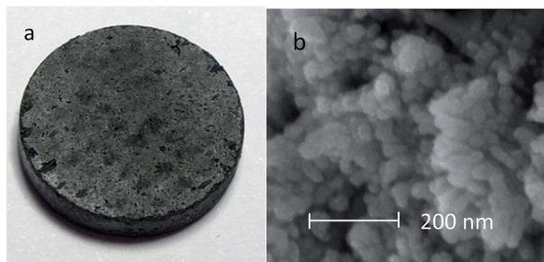
Fig. 4 (a)  $\text{Ta}_2\text{O}_5$  pellet collected after 80 min electrolysis in  $700$  °C MNK at  $2.0$  V. (b) Scanning Electron Microscopy (SEM) image of the Ta nanoparticles shown in (a) (after acid washing).
