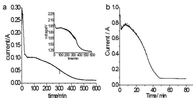
Fig. 2 Current–time plots of (a) potentiostatic electrolysis of a  $\text{Ta}_2\text{O}_5$  pellet in MNK at  $-0.8\text{ V}$  vs.  $\text{Ag}/\text{AgCl}$  and  $700^\circ\text{C}$ . Inset: corresponding cell voltage profile. (b) Constant voltage electrolysis of a  $0.7\text{ g}$   $\text{Ta}_2\text{O}_5$  pellet at  $2.0\text{ V}$  and  $700^\circ\text{C}$ .
