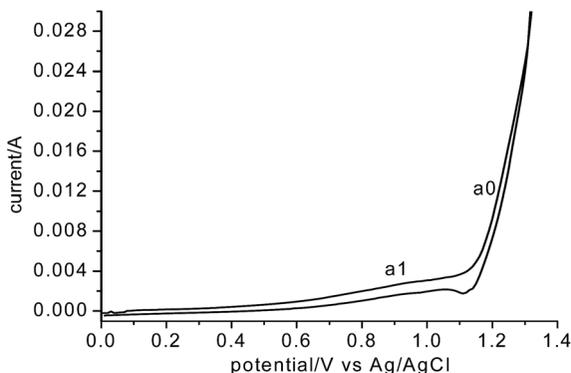
Fig. 7 Cyclic voltammogram of graphite in eutectic MgCl<sub>2</sub>–NaCl–KCl (700 °C) vs. Ag/AgCl, scan rate 200 mV s<sup>-1</sup>.
