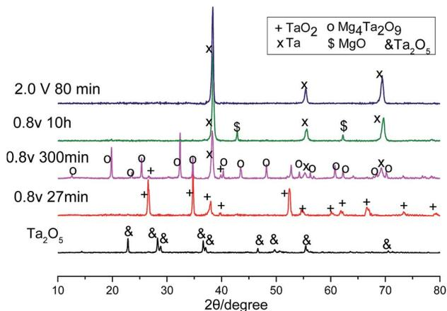
Fig. 3 XRD patterns of the products collected at the indicated times of potentiostatic electrolysis ( $-0.8$  V vs. Ag/AgCl, water washed only) and constant voltage electrolysis of  $\text{Ta}_2\text{O}_5$  ( $2.0$  V, water and acid washed) at  $700$  °C in MNK.
