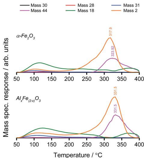
Fig. 4 TPD profiles of the haematite supports under linear temperature ramp, following methanol adsorption. The masses displayed correspond to HCHO (black), CO (red), CH<sub>3</sub>OH (blue), CO<sub>2</sub> (purple), H<sub>2</sub>O (green) and H<sub>2</sub> (orange).
