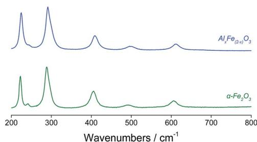
**Fig. 3** Raman spectra of Al-doped and phase-pure haematite.
