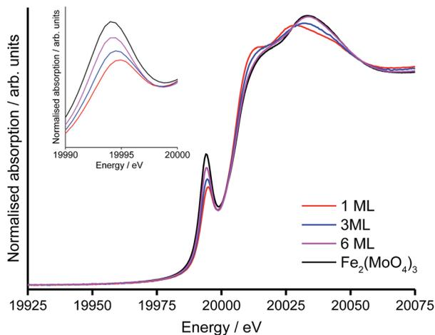
Fig. 5 Normalised Mo-XANES for 1, 3, 6 ML MoO<sub>x</sub>@HSA catalysts, including an enlargement of the pre-edge region.
